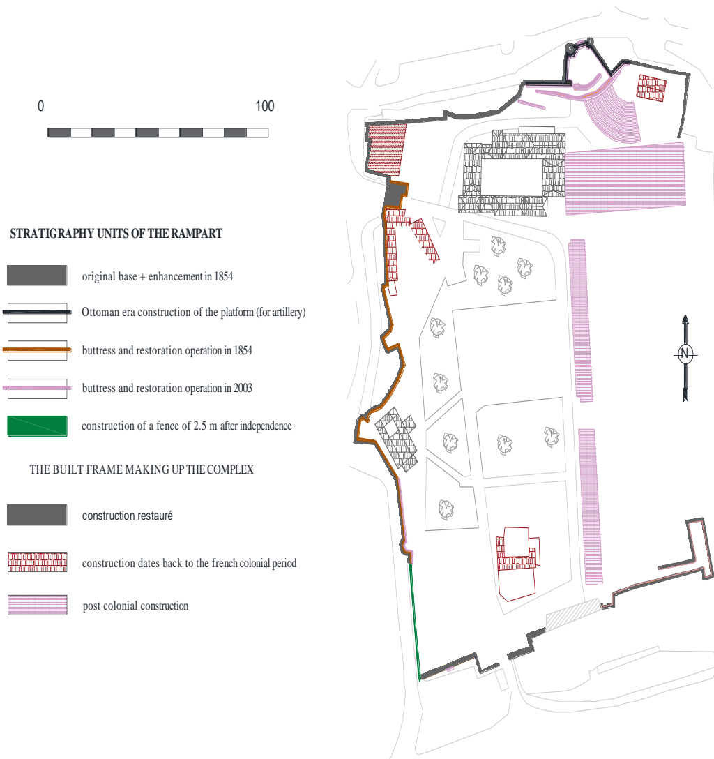
Fig. 9: Plan, a diachronic stratigraphic survey of the rampart of the El-Mechouar complex Source: authors
