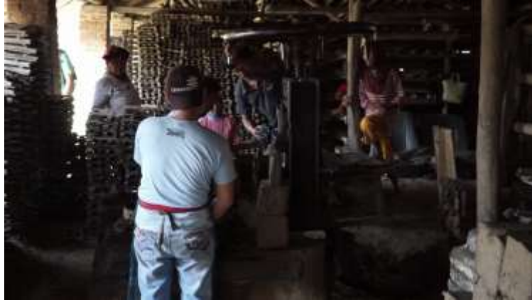
Fig. 5: Workers making roof tiles with a press machine in Jebor Herlang, Burujul Village Source: Author, 2019.
