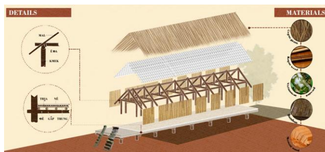
Fig. 7: Exploded diagram of the Longhouse structure Source: Students' illustration instructed by the first author, 2024
