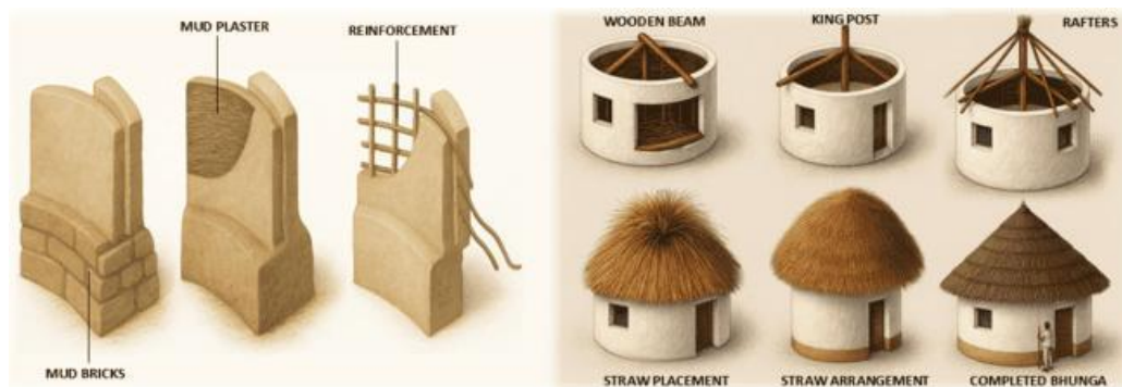
Fig. 12: Construction sequence of Bhunga houses in Kutch, Gujarat.
