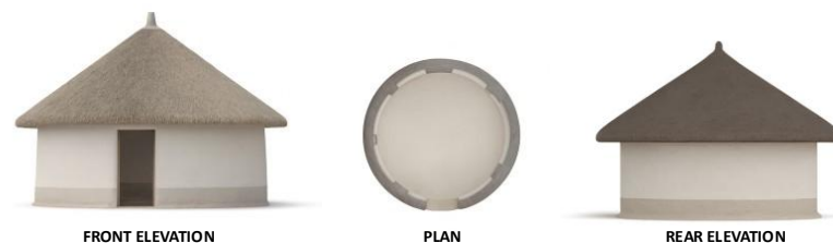
Fig. 17: Plan and elevations of a traditional Bhunga house in Kutch, Gujarat.
