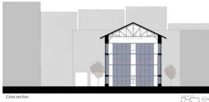
Fig. 8.1: Section of the Reference Section showing the 4-tier stacking system. Source: Author, 2024.
