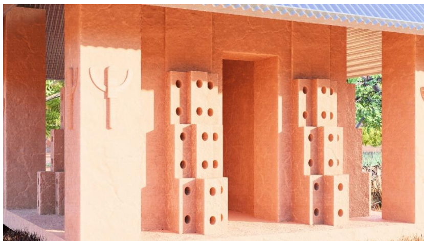
Fig. 20: Typical Buttresses on the central chamber of an illustrated model Source: Author, 2024
