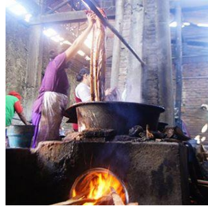
Fig. 9: The Wax Boiling Process Through Melorod by Dipping a Cloth in Boiling Water Source: Author, 2021
