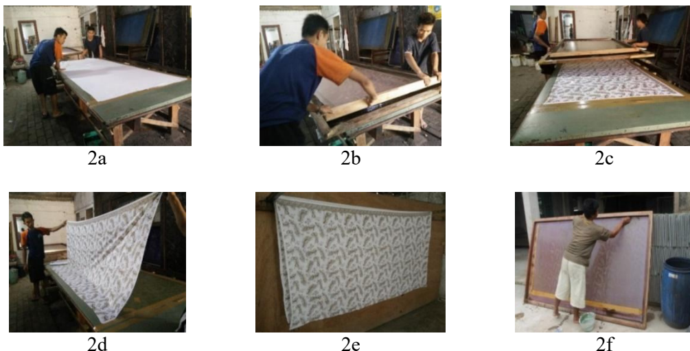
Fig. 2: Process Flow of Cold Wax Printing on Cloth Source: Author, 2021
