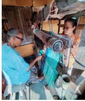
Fig. 4: The process of inserting warp threads into a gun eye.
