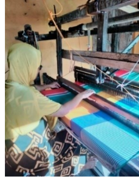
Fig. 5: Weft weaving on warp threads with ATBM tools.
