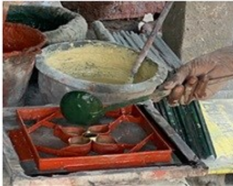
Fig. 4: Preparing the Coloured Mixes Source: Author
