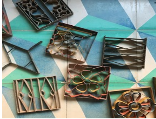
Fig. 9: Brass Stencil for tile making, Athangudi (Source: Author)
