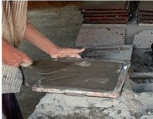
Fig. 6: Filling of tile with a layer of cement mortar Source: Author
