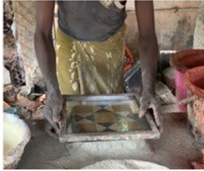
Fig. 3: Step 1 - Preparing the Stencil Source: Author
