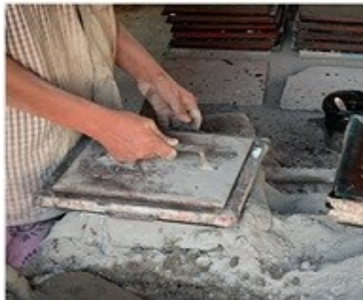
Fig. 7: Leveling and compressing the surface of the tile Source: Author
