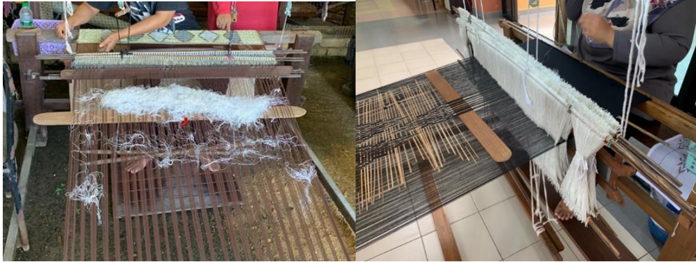
Fig. 5: The use of traditional “Karak” and 'heddle eye' on a loom- Source: author
