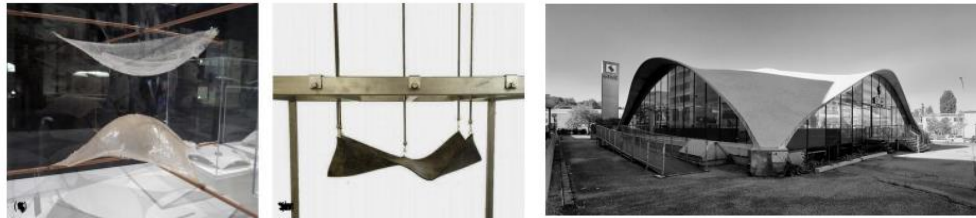
Fig. 4: Suspended models: suspended model of wooden structure, cloth and Heinz Isler ropes (Grieco, 2012); equipment for the production of structures based on the form-finding technique Source: Gáspár, 2020. Pavilion of Sicily in Genoa. Heinz Isler (Jyhem, 2013)
