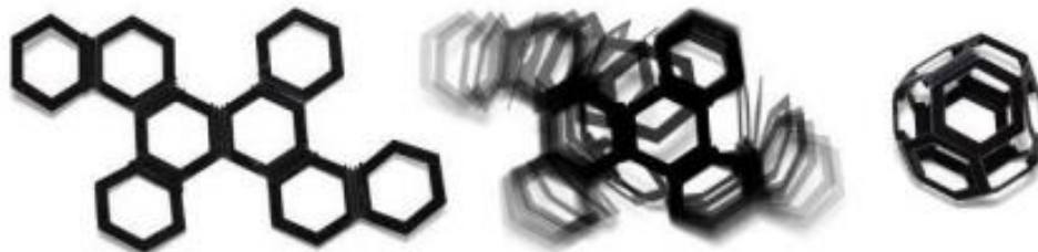
Fig. 11: The transformation of a planar structure manufactured by 4D printing for a truncated octahedron (from left to right) Source: SelfAssembly Lab / MIT, n.d.
