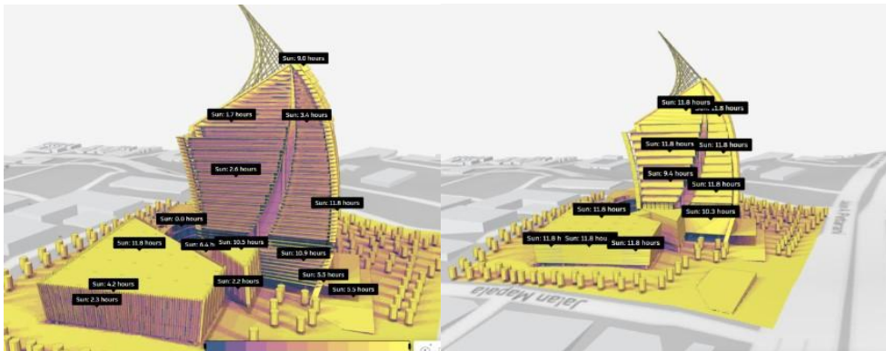
Fig. 6: Simulation on June 22 northern side of the building with and without shading Source: Author, 2023
