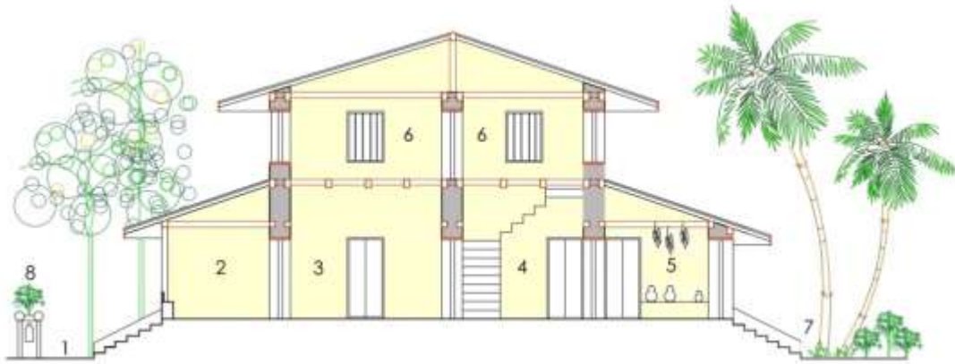
Fig.8.c: Schematic section of House influenced by Socio-economic status at Sawantwadi. 1. Aagan 2.Loota 3.Majghar 4.Majghar (for female) 5. Padavi 6. Mala (Attic) 7.Paras 8.Tulsi Vrundhavan Source: Author
