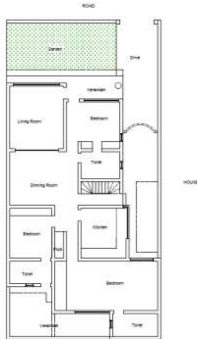
Fig. 8: Ground floor plan of contemporary residence at Greater Kailash Jammu Source: author
