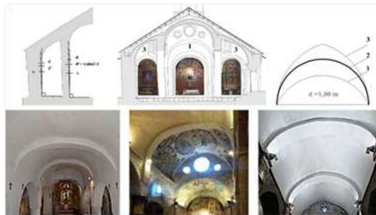
Fig. 11. Study of the typology of vaults. 1) Relation < 1.57 ; 2) Relation = 1.57 ; 3) Relation > 1.57 .
