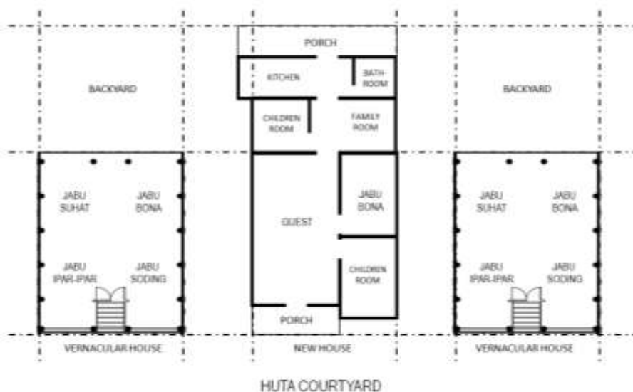
Fig. 11: Spatial Order of New House (center) Flanked by Vernacular Houses
