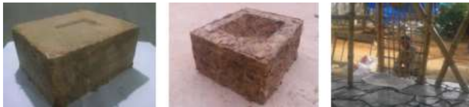
Fig.15: Stabilised Bamboo Fibre (left) and Bamboo, Newspaper waste (centre) mud blocks Source: Author
