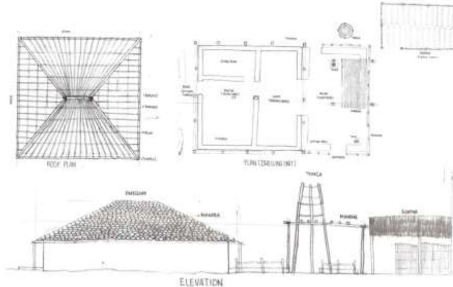
**Figure 2:** Dwelling unit plan, roof plan and elevation of bhariya tribe at Patalkot
