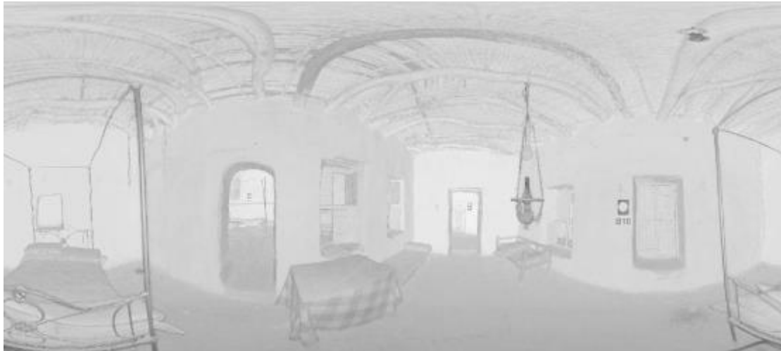
Fig. 3: Laser scanning measurements used as experimental measuring tool in Balat. One can get accurate measurements for vernacular buildings compared to manual sketches.
