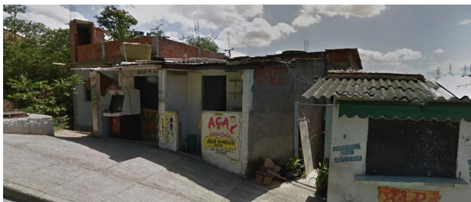
Fig. 8a. Construction Type 1 with corrugated tin directly on a load-bearing wall. Complexo do Alemão. (Source: Google Streetview, May 2015)
