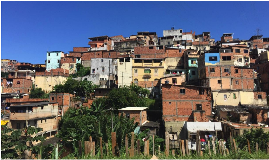
Fig. 6. Favelas of Salvador, Brazil, with reinforced concrete structural frame and structural clay tile infill walls
