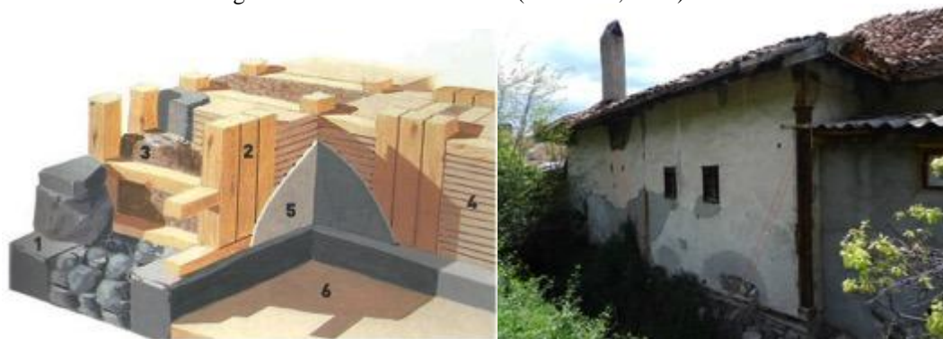
Fig. 17: Reconstruction of the walls in Great Temple, 1: Foundation and socle stone blocks; 2: Timber framework; 3: Filling of earth and stones; 4: Mud bricks; 5: Wall plaster; 6: Lime-plastered floor on a layer of packed earth (Source: Seeher, 2011) Fig. 18: Prop Structure of Özelevi (Source: author)
