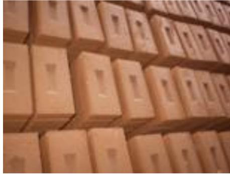
**Fig. 2:** Compressed Stabilised Earth Blocks
