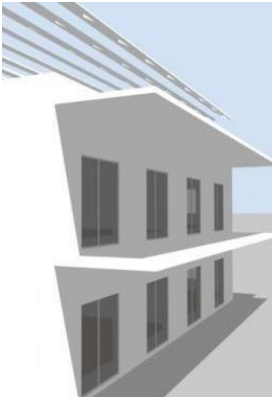
Figure 9. Shading of the south façade with deep eaves
