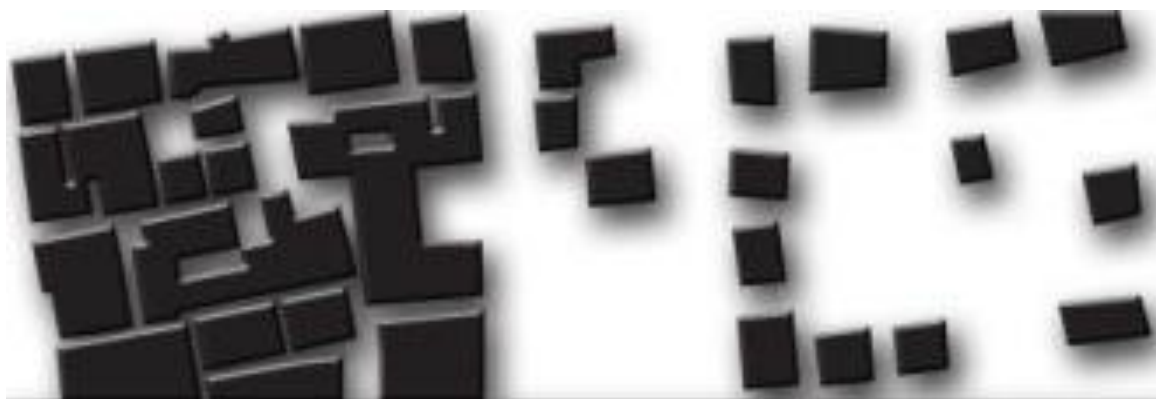
Figure 2. Illustration of the shading effect of built structure in Kumbahçe region of Bodrum (Not to scale). On the left, old patterns in the city centre. On the right, the settlement patterns of the tourism era. Note the differences between the shading affect through streets and the densities of the buildings.
