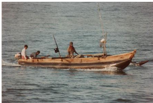
Fig. 14: Outboard motor on transom stern of a mechanized vallam oru
