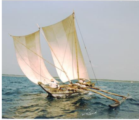
Fig. 9: oruwa seagoing outrigger craft Source: Kapitan, G.
