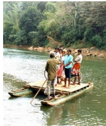
Fig. 6: añgula twin-hulled ferry Source: Kapitan, G.
