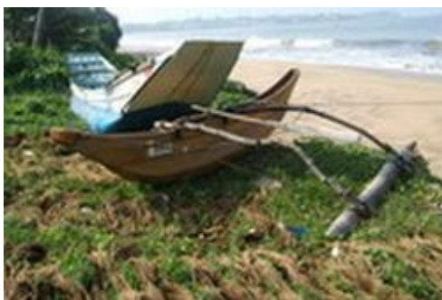
Fig. 15: Small oru with hull and washstrakes moulded as one. Behind: a mā-dāl-pāru of GRP Source: Grainge, G
