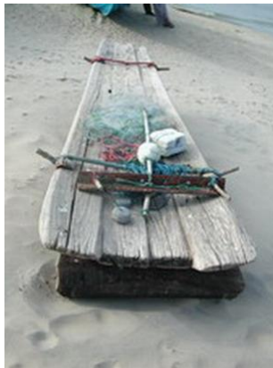
Fig. 5: teppam pegged-log raft Source: author
