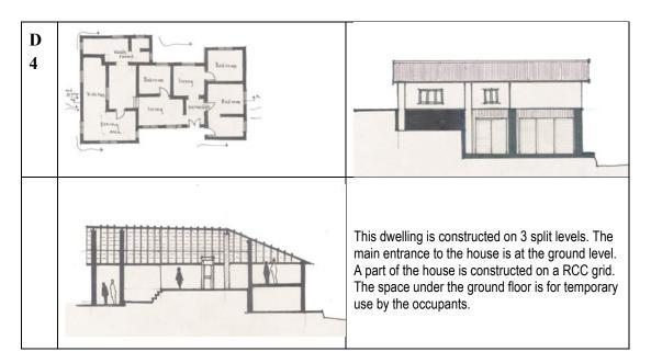
It is noted that the majority of the houses observed had been constructed at the highest practical location, with raised plinths above the highest flood levels known. Longer walls were parallel to flood flow and most houses also had a storage and evacuation attic. The roofs were always above the flood level and... Nevertheless, none of the walls have been braced by cross walls or continuous lintels.
