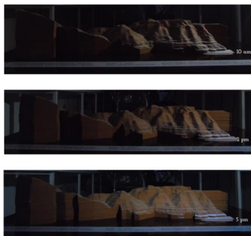
Fig. 29: Site hill shade analysis using a physical model of the hill site Source: Author
