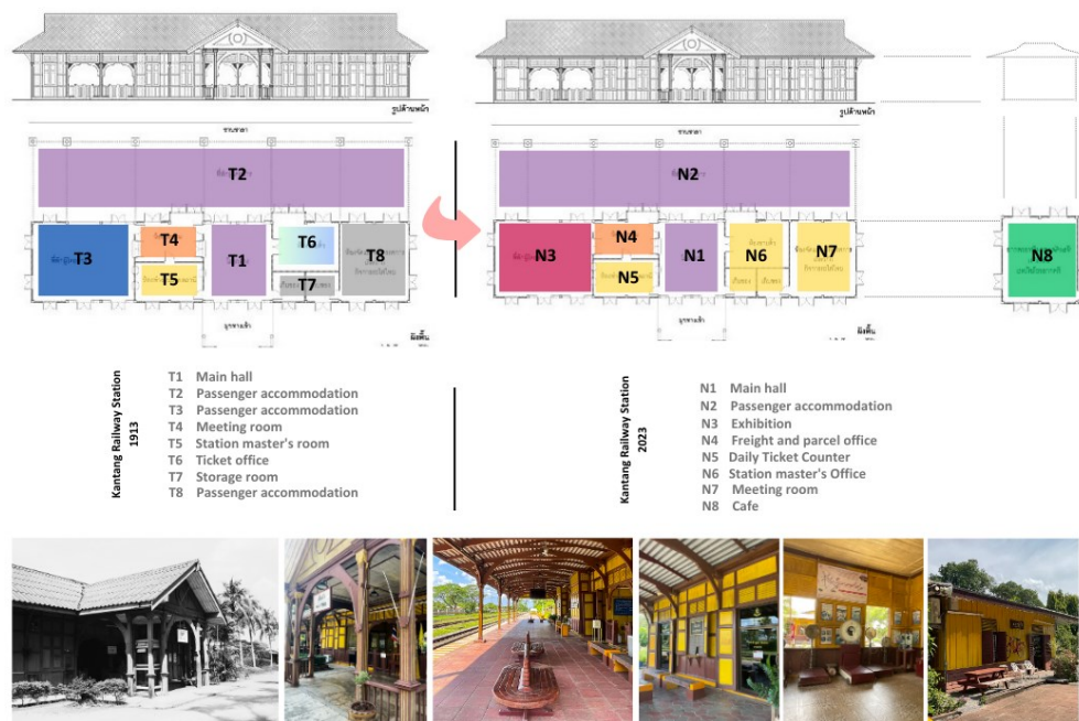
Fig. 7: Transforming Kantang Railways Station into Kantang Train Exhibition and Café. Source: Author (modified from Construction drawings the State Railway of Thailand, 2023)
