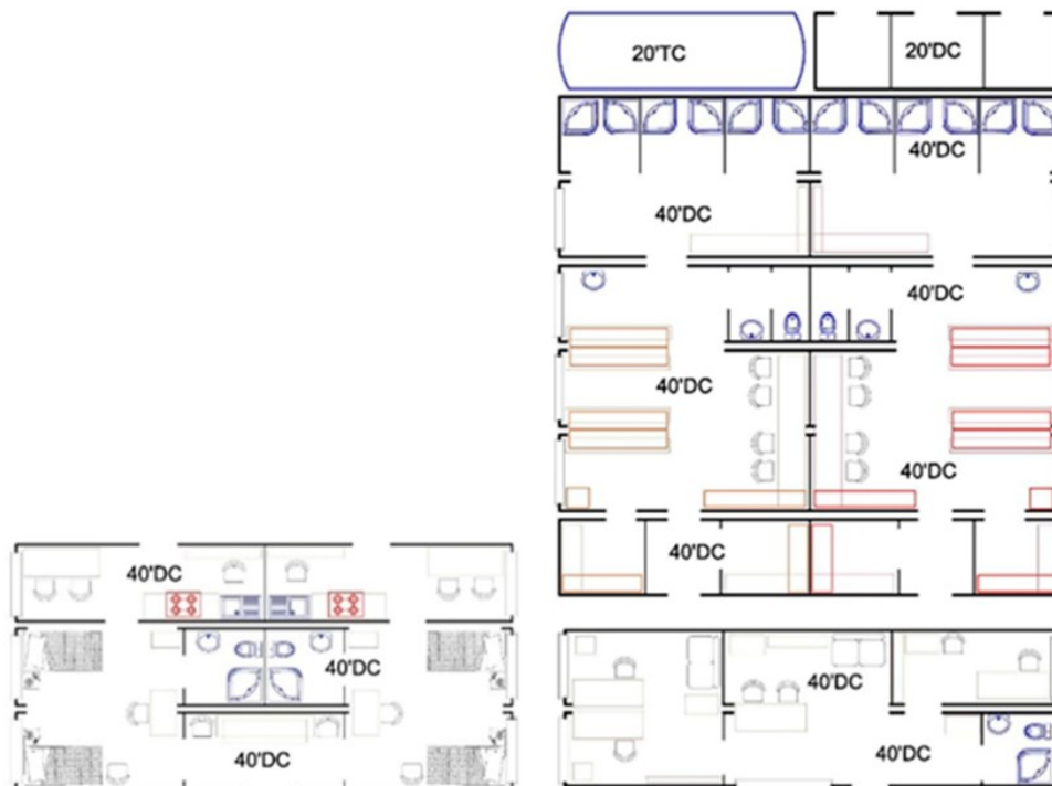
Fig. 10: The template of the combination of the administration pavilion, on-duty staff resting pavilion, and pavilion of staff amenity rooms
