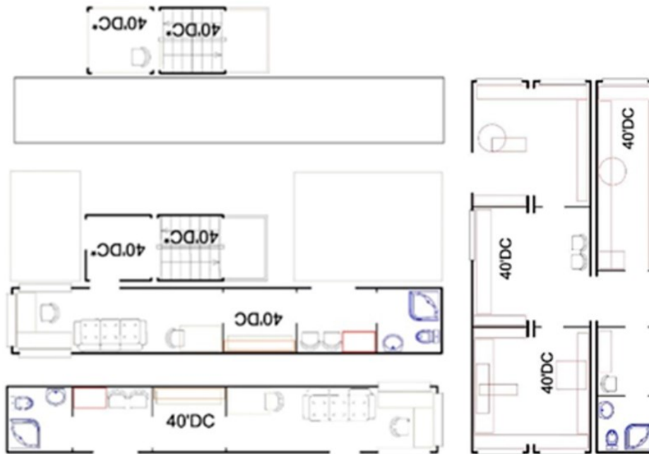
Fig. 8: The template of the combination of security room with check point and the repair shop Source: Author
