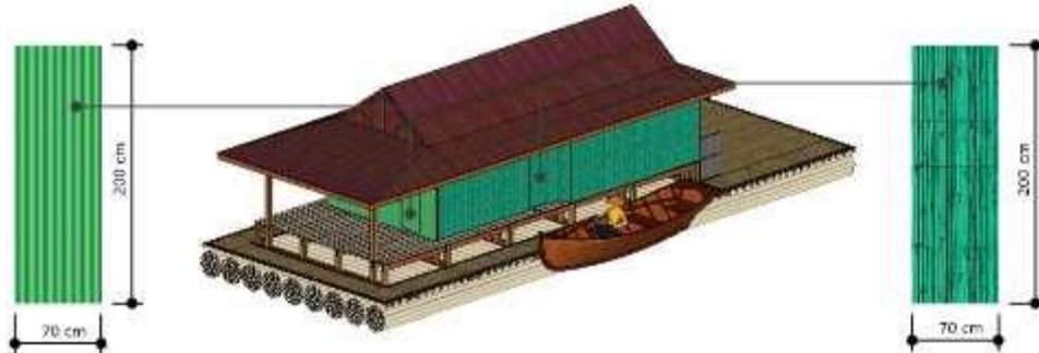
Fig. 13: The location of the large floating house door Source: Sari, 2023
