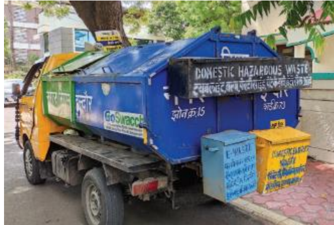
Fig 2: Compartmentalized vehicle for collection of biodegradables, non-biodegradable, sanitary, household hazardous and electronic. Source: Alappuzha (2021)
