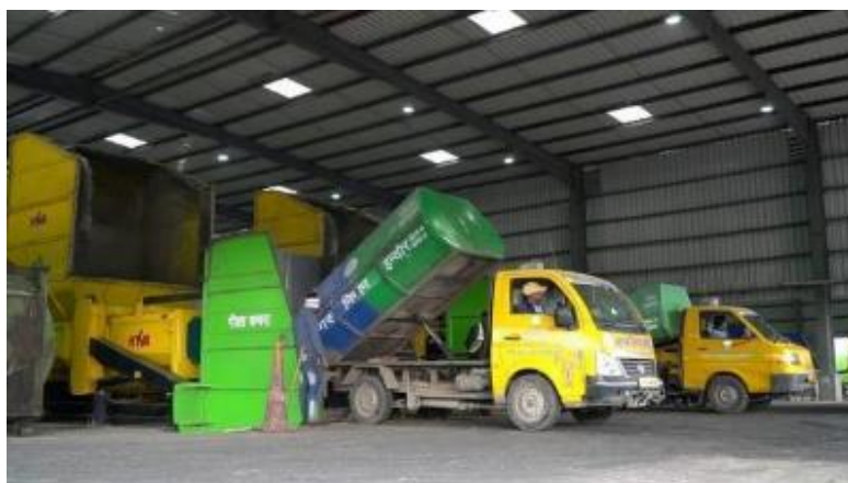
Fig 6: Divided Tipper for wet and dry waste collection. Source: https://www.smartcityindore.org/solid-waste/
