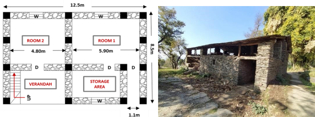
Fig. 9: Typical Rectangular Floor Plan with openings in walls for ventilation Source: Kant and Kumari, 2021
