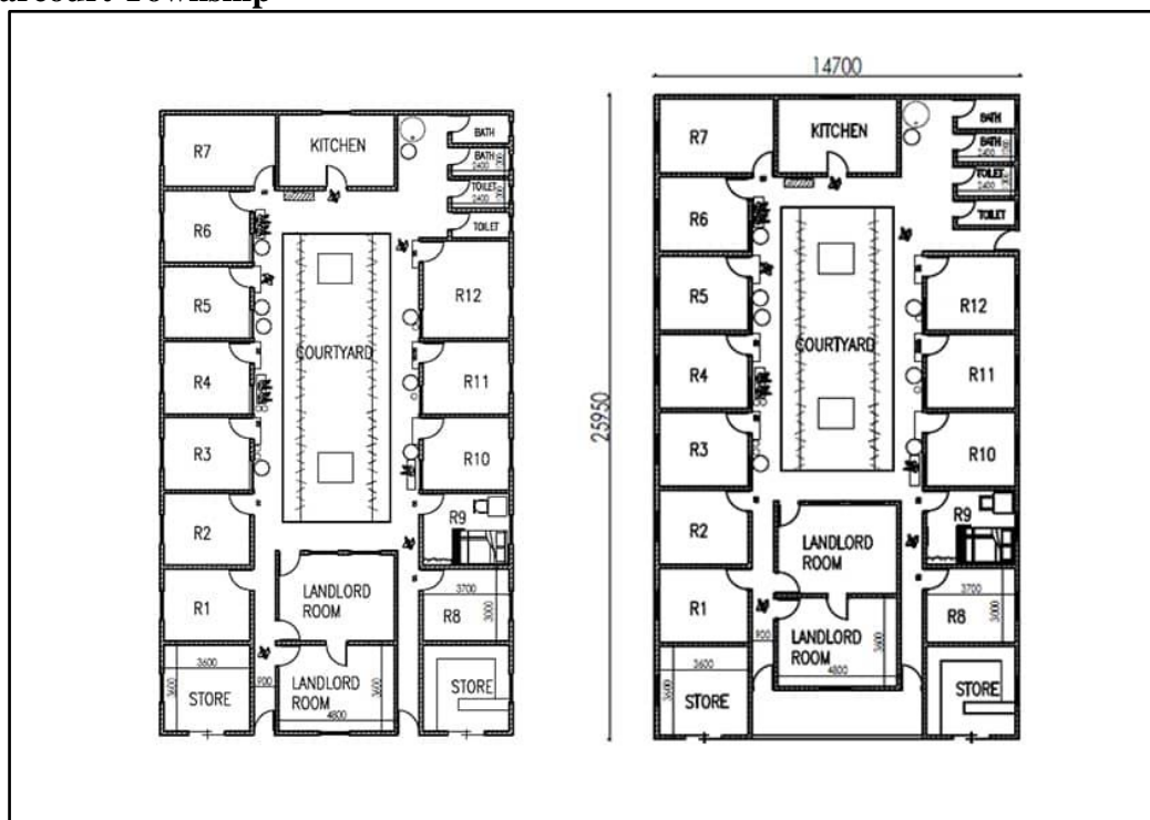
Fig. 4: Typical floor plans showing differences in design between bungalows in Diobu and Old Port-Harcourt Township
